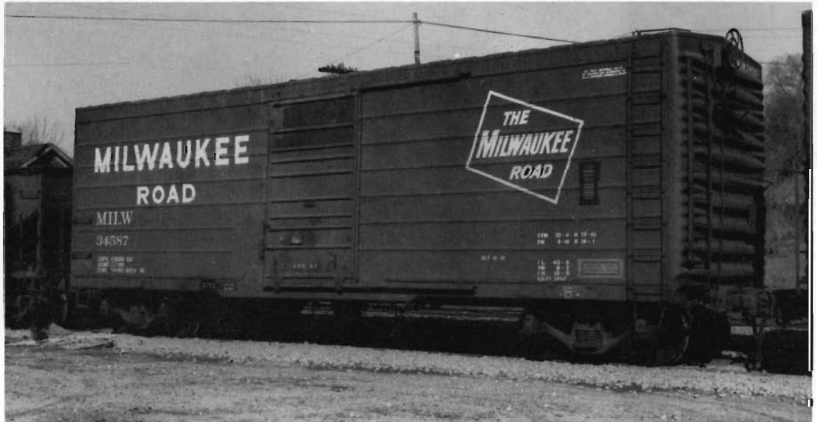
MILW 34587. An original production version of the 40' box, this 10'6" car was photographed in March 1971 outside Camden, AL. Note the full length ribs, Camel door, 8-run ladder and Dreadnaught 5/5 end. (H.W. Ameling collection.)
