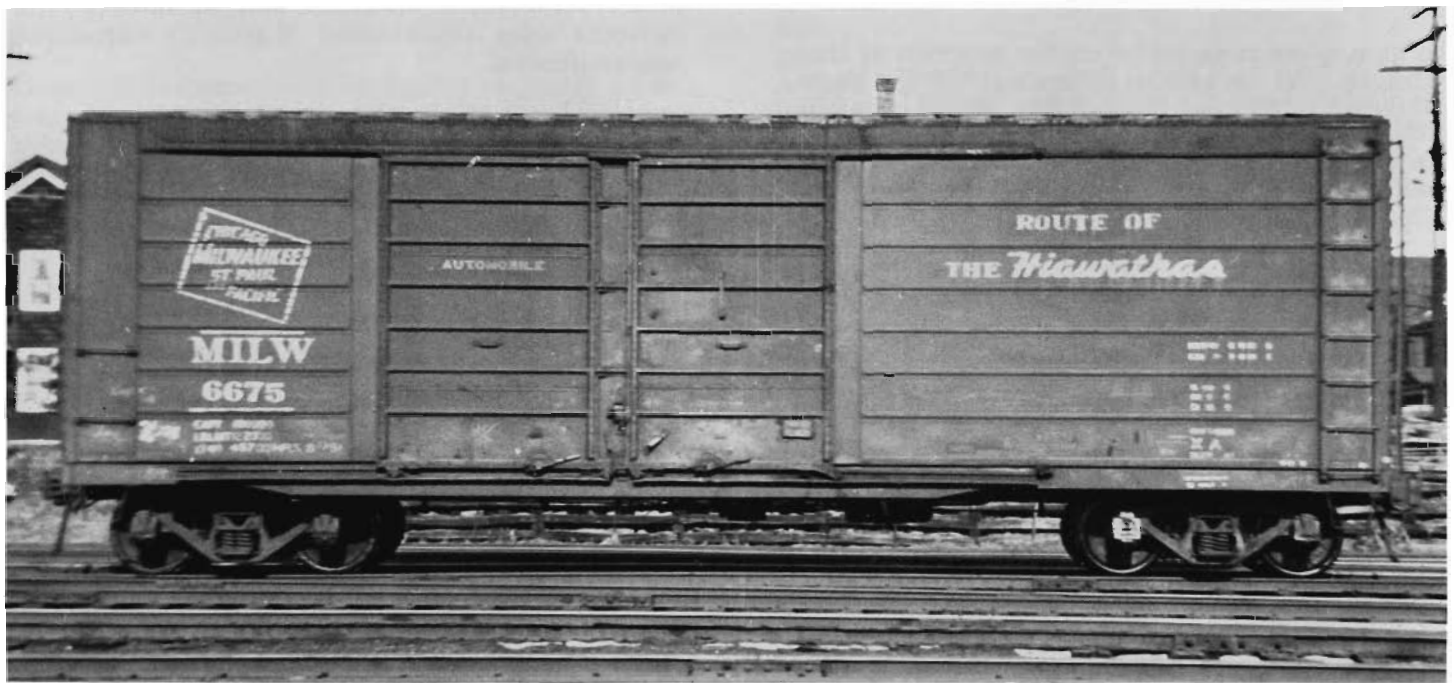
MILW 6675. A double door 40' automobile box car. The 8-rung ladder reveals that this is 10' 6" car. The older style rhomboid logo was applied to the left end of these cars because there wasn't enough room to apply "The Milwaukee Road." (C. K. Yungkurth, Rail Date Services .)
