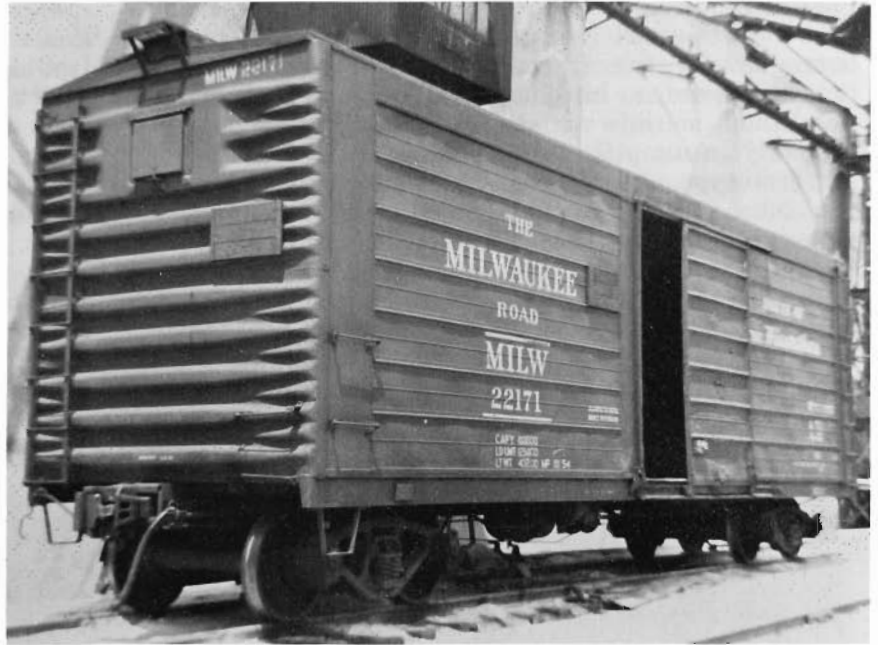
MILW 22171. Photo taken on the NKP in Zanesville, OH clearly shows the "mid-rib" design. (R.C. Feld photo; collection of John C. LaRue, Jr.)
