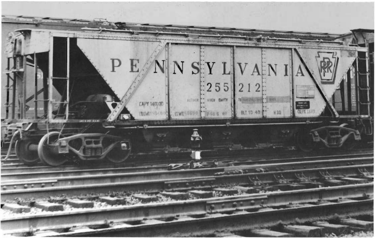
PRR 255212 is an H30 built in 1940, carrying the 1950s paint scheme and photographed in the early 1960s. The unique “truss bridge” side bracing and the car’s low profile versus the other cars in the scene are evident.
